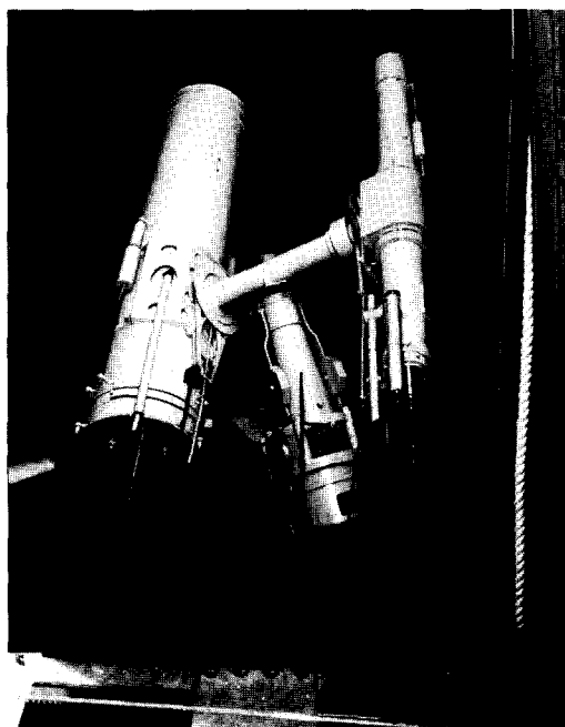
The 1885 Isaac Roberts twin equatorial telescope was in store for 20 years before being overhauled for use at Herstmonceux. It was used there for four years before installation in the Science Museum's observatory.
